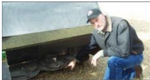
Figure 3. Adjust cutterbar gauge shoes so that stubble height is 4 to 6 in. to help trap snow and improve winter survival
