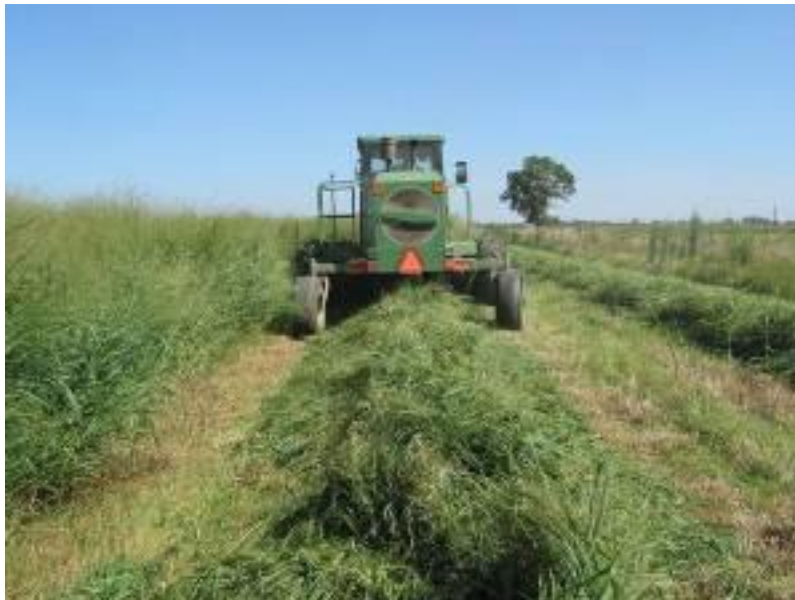
Figure 1. Rotary head mowers (disc mowers) effectively harvested this 6-ton per acre switchgrass.
