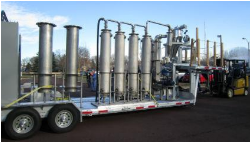
Figure 1. This skid-mounted pyrolysis system, developed at the USDA Agricultural Research Service, can process two tons per day of biomass. Photo Credit: USDA ARS.
