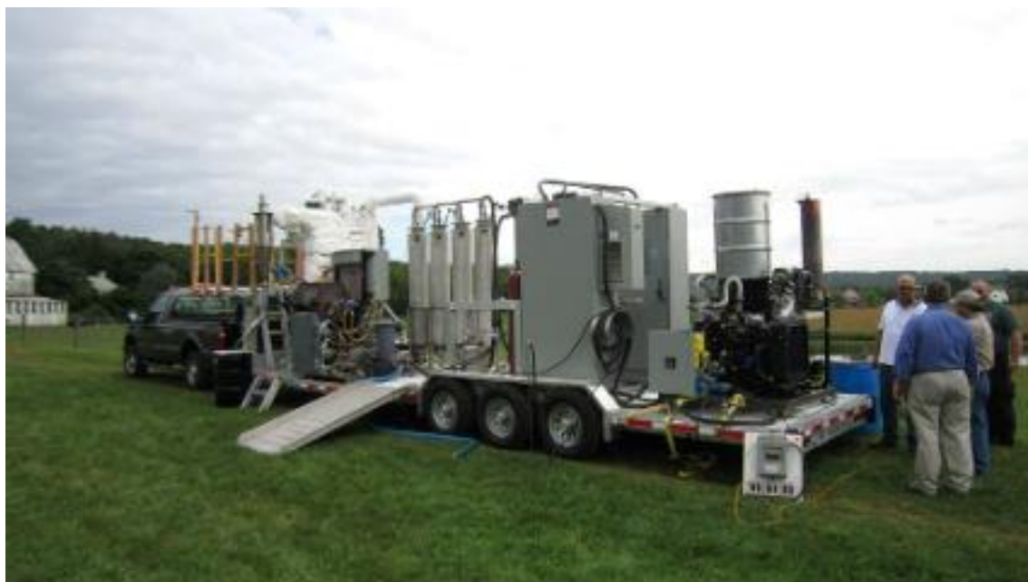
Figure 1. FarmBio3 mobile pyrolysis system travels among farms simulating the real-world scenario of multiple on-farm units that convert feedstocks to bio-oil, which is delivered to a regional biorefinery.
