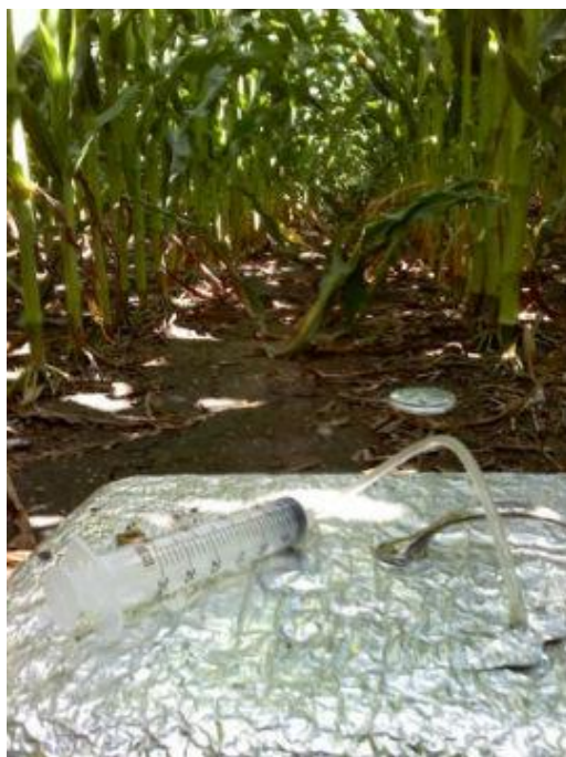
Figure 2. Static chamber used in research. Photo: Virginia L. Jin.
