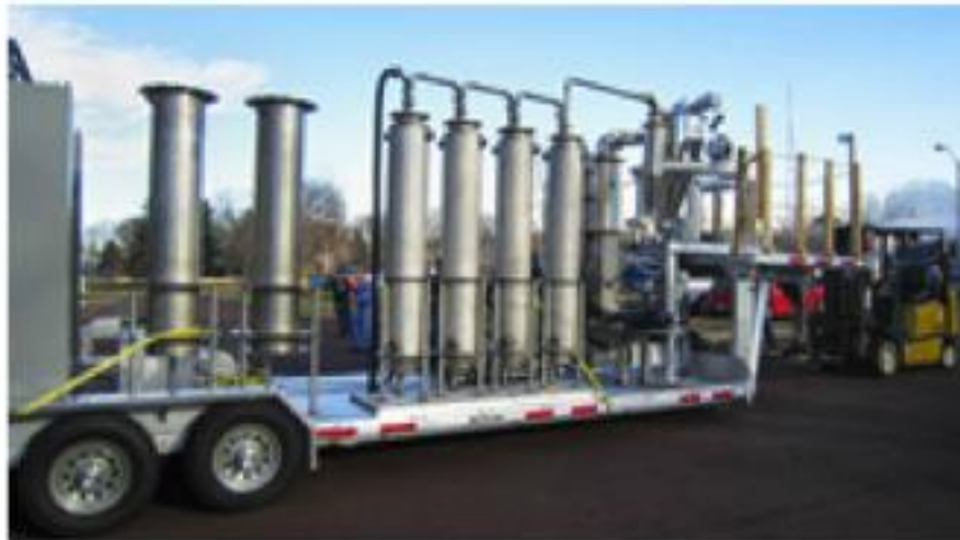
Figure 4. Prototype mobile pyrolyzer. Photo: Akwesi Boateng, USDA ARS
