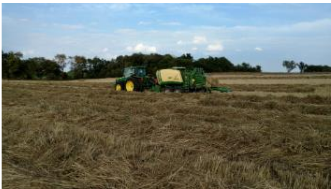
Fig 3. The Logistics Team evaluated how much energy a commercial, high-density, large-square baler uses when making bales of greater density, critical to efficient transport of bales. Photo: Kevin Shinnars, University of Wisconsin
