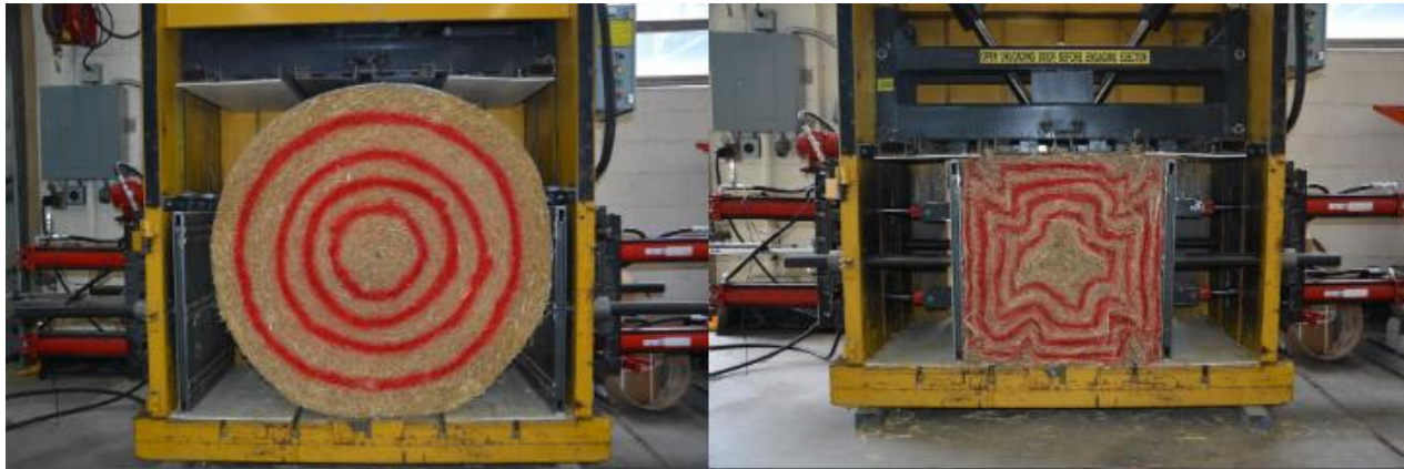
Figure 4 . The Logistics Team designed this recompression press to increase the density of round
