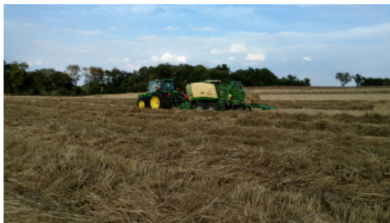
The Logistics Team evaluated how much energy a commercial, high-density, large-square baler uses when making bales of greater density, critical to efficient transport of bales. Photo: Kevin Shinnars, University of Wisconsin.
