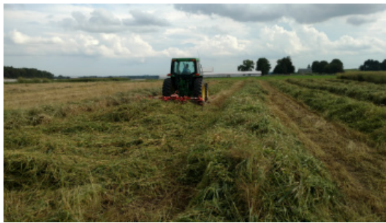
Tedding a switchgrass crop mowed in wide swaths speeds drying. Photo: Kevin Shinnars, University of Wisconsin.
